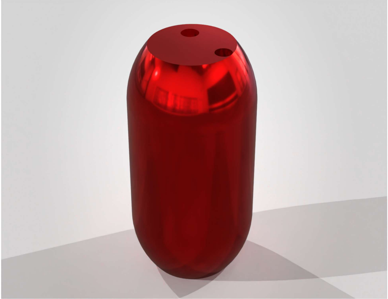
Figure 6: Rocket fuel tank. Two orifices are used to adapt to input requirements of the turbopump
