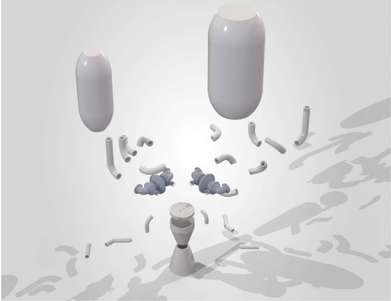
Figure 11: Exploded view of the electric pump-fed liquid rocket engine assembly
