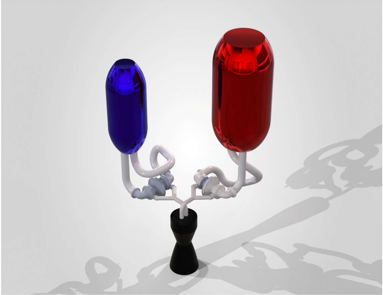
Figure 10: Isometric view of the electric pump-fed liquid rocket engine assembly
